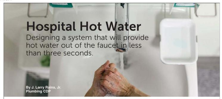
ave you ever wanted to design a domestic hot water system that worked — one that provided 105- to 110-degree hot water in two seconds after the faucet was turned on, that does not use balancing valves and, best for last, is cheaper to build when compared to the traditional two pipes (hot and hot water return system) installation? Welcome to Jump Routing.
